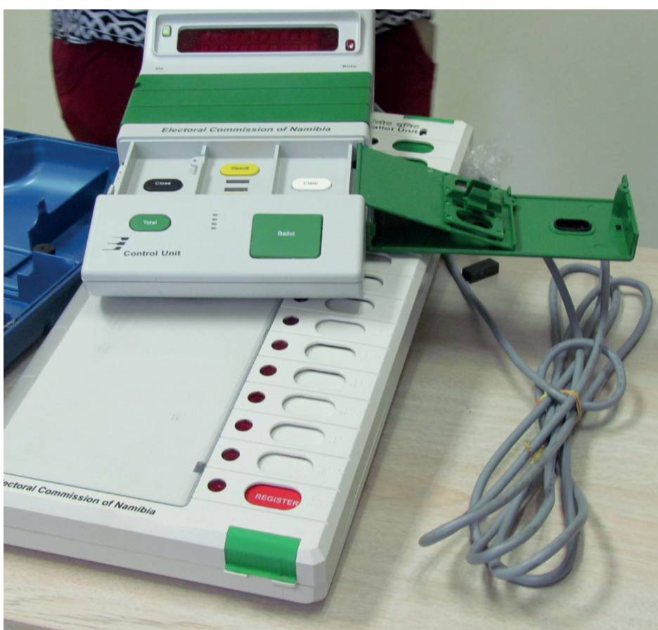
An EVM consists of a control unit and a ballot unit
